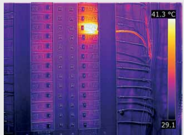
Detect loose connections and other defects in high, medium and low-voltage electrical equipment
